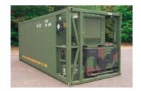
Description: Consists of a 9,000 BTU refrigeration unit and 8'×8'×20' ISO insulated container, with approximately 800 ft<sup>3</sup> of usable storage. The refrigeration unit is electric and can be set for refrigeration or freezer temperatures. A 10 kW Tactically Quiet Generator (TQG) is mounted within the envelope dimensions of the container to provide electrical power for the unit and lighting inside the container.
